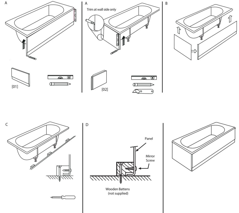
Should the cutting of panels be necessary (due to water pipes or skirting boards) a small fine toothed saw or sharp knife is recommended.
